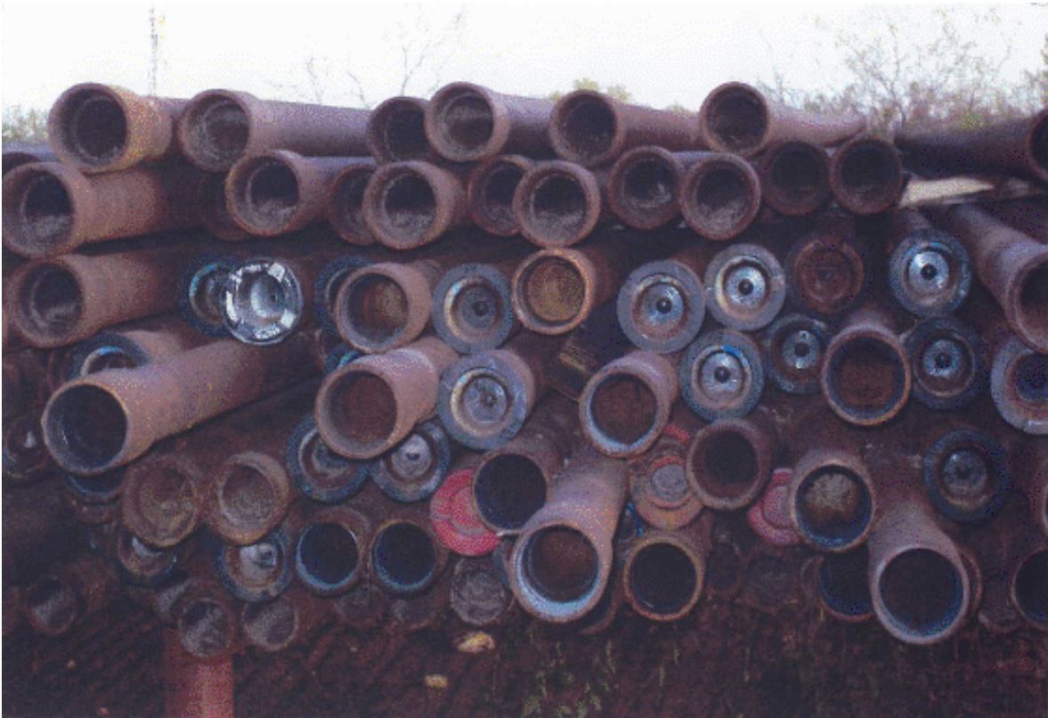
Pile of used gas pipes with NORM build-up (scale) in Texas. Photo credit: Marvin Resnikoff
